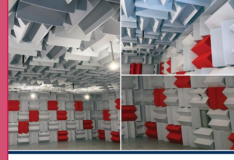
maintaining a low noise floor inside the chamber with minimal profile that no other noise control product supplier can match.
